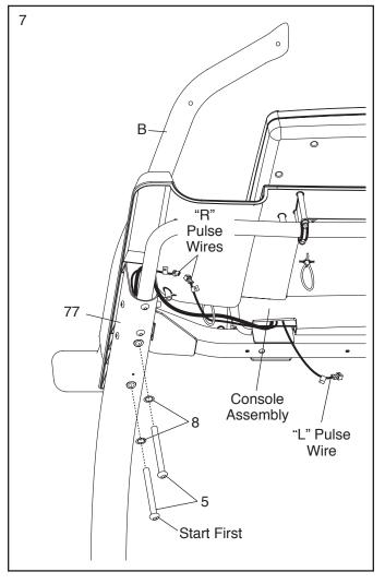
8. Hold the left handrail assembly (C) near the left Upright (77). Insert the pulse wire from the left handrail assembly into the hole in the top of the Upright and out of the end of the Upright.
